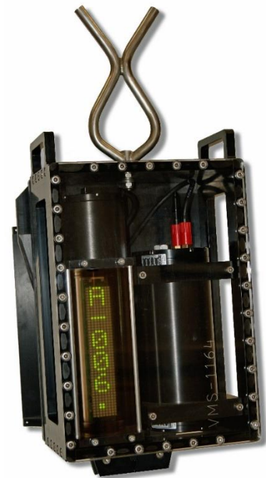
DISTIL-V, shown here as part of a VMS verticality measurement package
