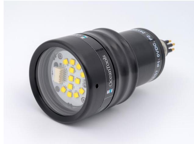
The OceanTools **L4** subsea light utilises high density LED technology with 80-CRI colour accuracy and 6500K colour temperature as standard. It generates a wide angle flood beam and achieves an impressive output of up to 10,000 lumens from a surprisingly compact 4000m depth rated package.
