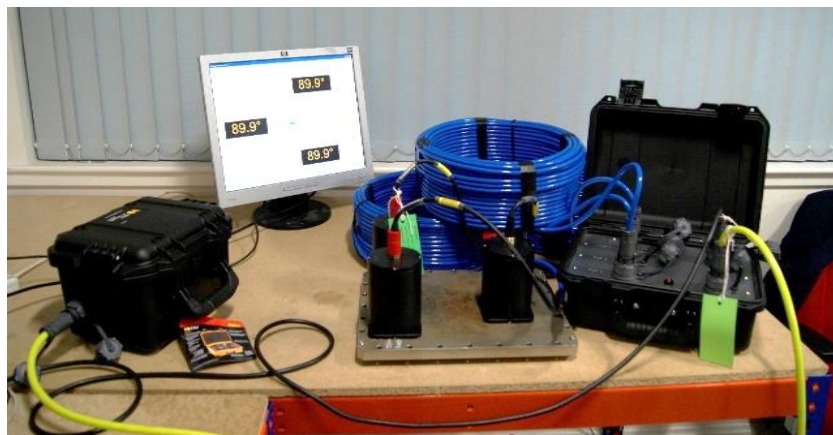
System of 3 sensors undergoing a bench test
