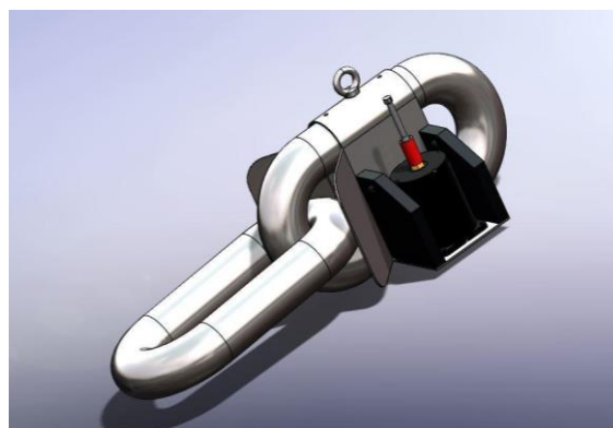
Typical mooring chain mounting bracket
