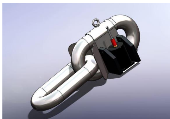
Typical mooring chain mounting bracket
