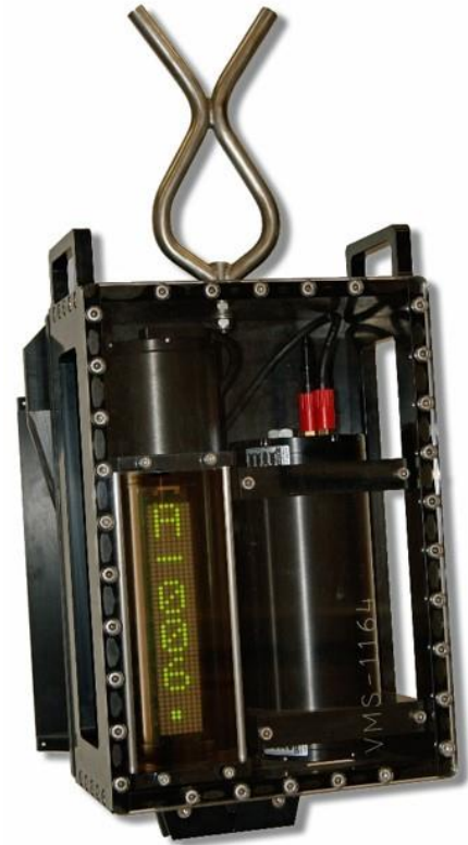
DISTIL-V vertical inclinometer display, shown here as part of VMS verticality package
