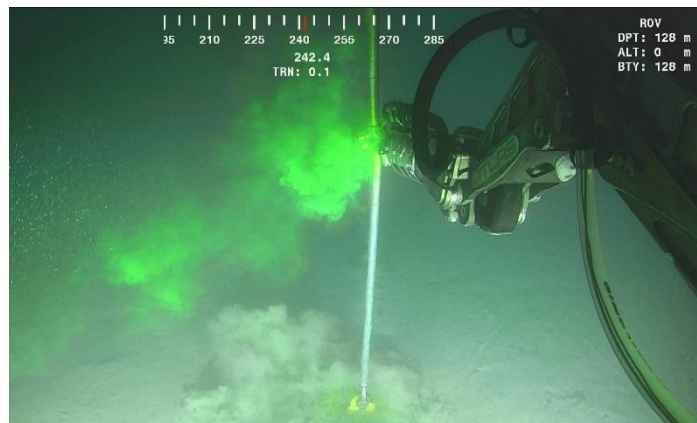
Cement detection with a DyeTector
